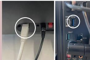
\*Note: For desktop computers, be sure to connect the USB 3.0 port on the back of the host computer.
